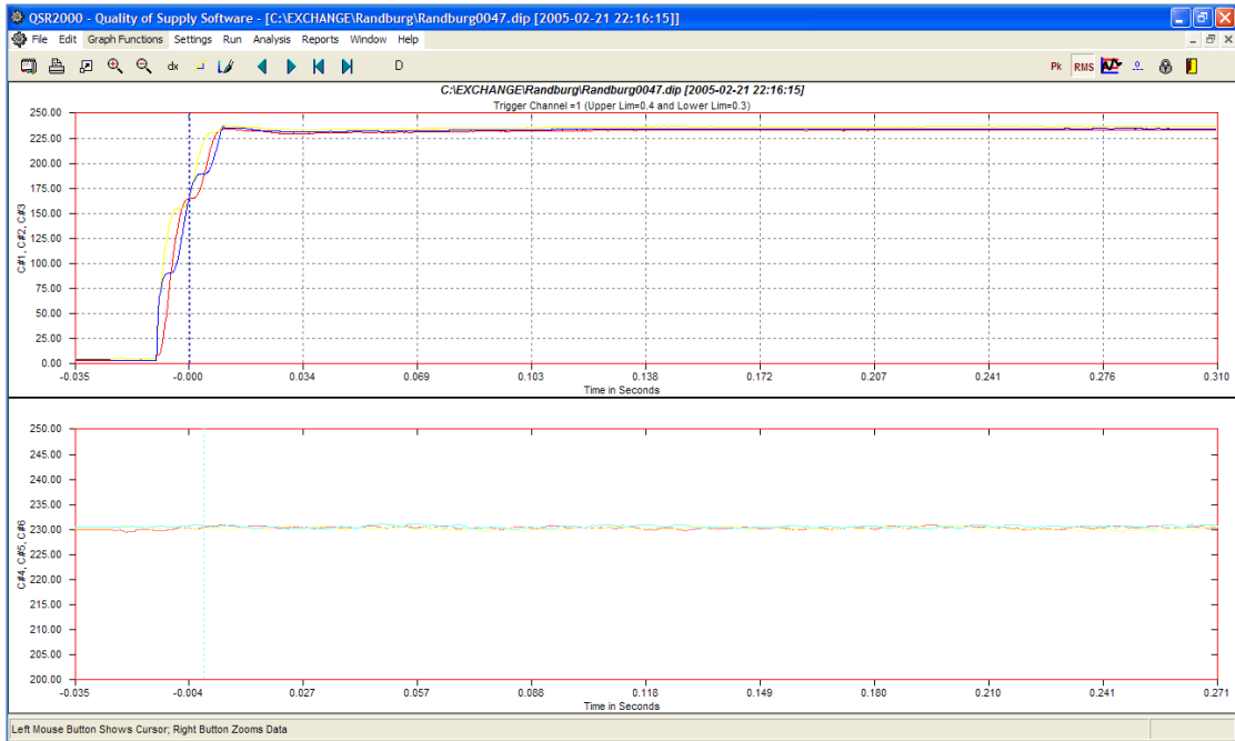
Figure 15: Incoming Supply Restored with Corresponding UPS Output
