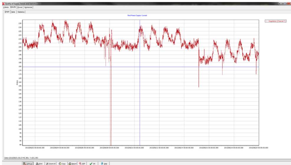
Figure 21: Substation Current Profile for Data Centre Loads
