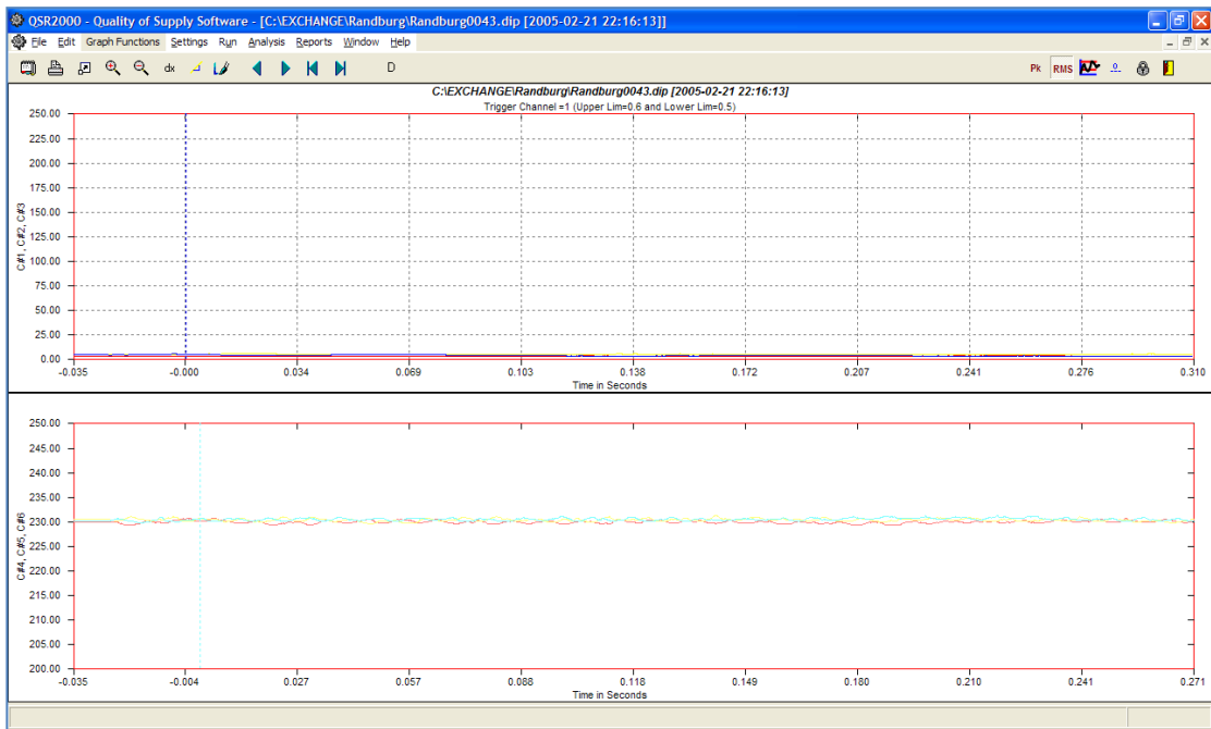
Figure 14: Incoming Supply Failure with Corresponding UPS Output
